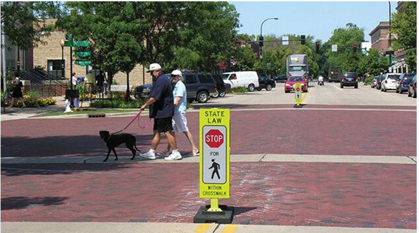
Paddle signs in the middle of Market Street will better alert motorists to the crosswalk and will also encourage slower vehicle speeds.
